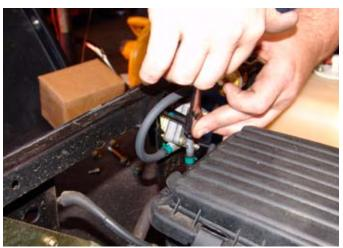
**STEP 8:** Un-bolt fuel pump and save the bolt.
