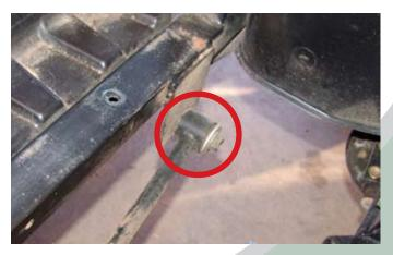
**STEP 9:** Un-Bolt the panhard bar and save the nut and bolt.
