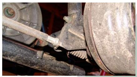
**STEP 4:** Remove both left and right brake lines from the brake drums.
