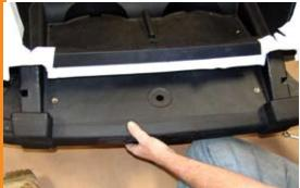
**STEP 7:** Remove the rear bumper and save the side bolts for use during installation.
