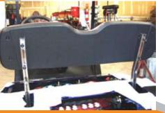
**STEP 5:** Install the front seat back using OEM bolts.
