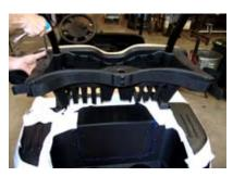
**STEP 3:** Remove the 4 bolts to the top supports and remove the top supports.
