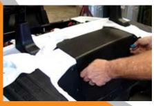
**STEP 5:** Then remove the inspection cover and front seat for access.
