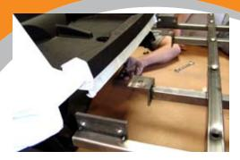
**STEP 2:** Take the OEM bolts removed from the bumper and bolt the step frame into place with the side tabs facing up.
