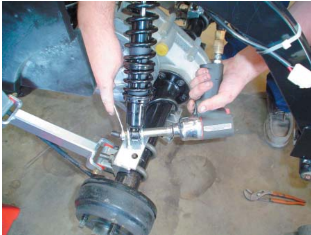
STEP 5: Tighten shock bolts.
