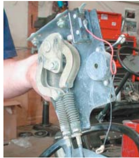
STEP 11: Take passenger side shifter cable and remove dust boot and adjuster nuts.
