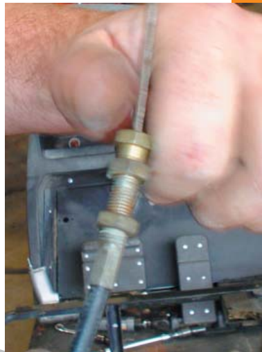
STEP 11: Take passenger side shifter cable and remove dust boot and adjuster nuts.
