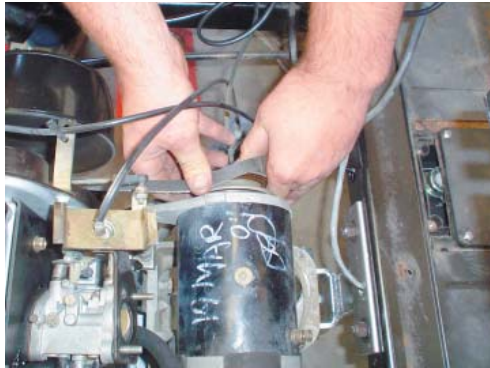
STEP 3: Reinstall starter belt.
