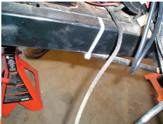
STEP 12 Cable tie brake line to car frame up to 1999 models.
