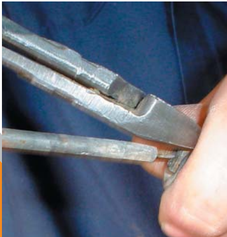
STEP 11: Take passenger side shifter cable and remove dust boot and adjuster nuts.
