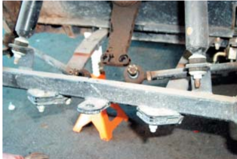
STEP 9: Disassemble the inner tie rod assembly.
