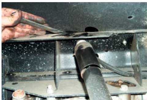
STEP 11: Using access holes under the front end remove the stock shocks.
