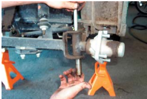
STEP 10: Remove stock king pins.
