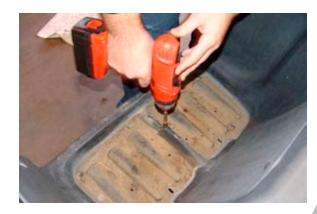
STEP 6: Using a 5/16 drill bit drill out the bolt holes to accept new bolts for the seat kit.
